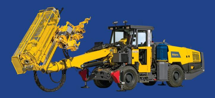
The **Diamec Smart 6M** from Epiroc combines the best of two worlds – the high productivity and accuracy of a **Diamec** core drilling rig, with the mobility of a well-proven, robust carrier designed for underground use.
